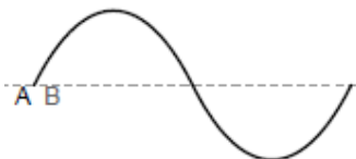
Phase shift = 0 degrees A and B waveforms are in perfect step with each other
