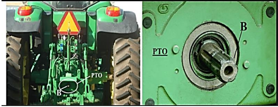
The position of the PTO and PTO's drive shaft (B) on a farm tractor
